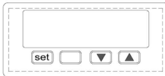
picture 2: Digital display for adjusting the temperature of the washing solution, located on the machine control panel
